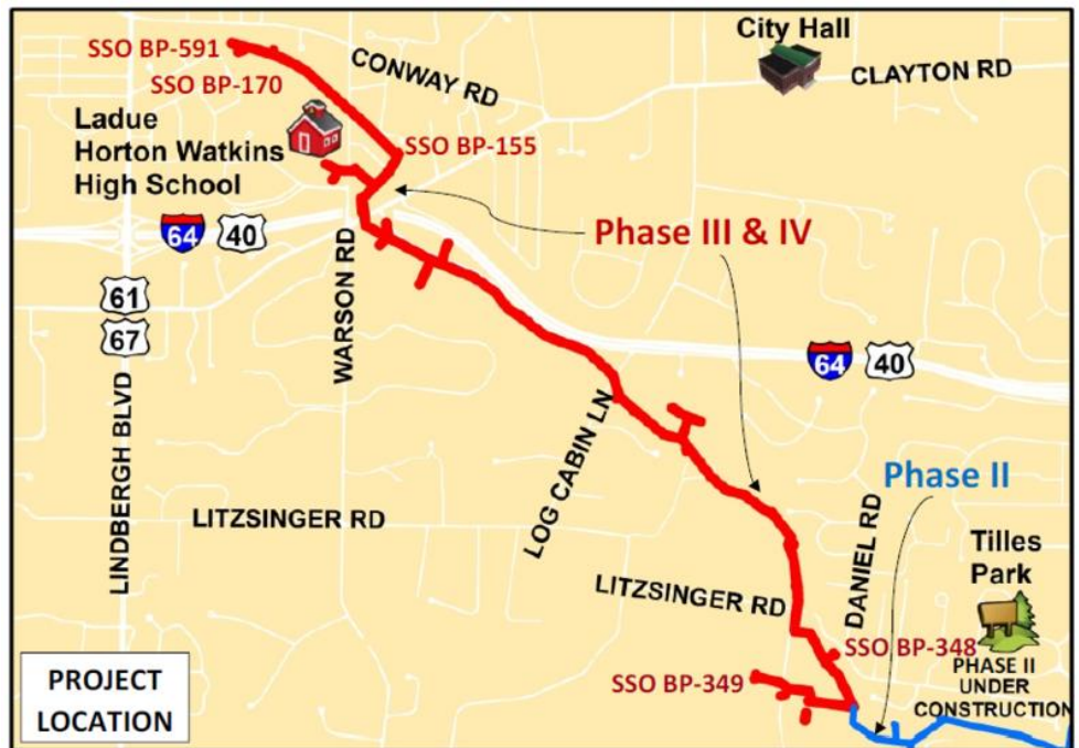
The Metropolitan St. Louis Sewer District began September 2019 to build a 3.2-mile sewer line in Ladue. ---CREDIT METROPOLITAN ST. LOUIS SEWER DISTRICT
